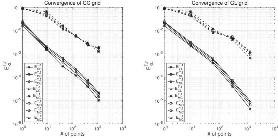
Figure 4: Convergences of the solutions computed over the CC grid (left) and over the GL grid (right). The dashed lines in both graphs represent the MC simulations.
