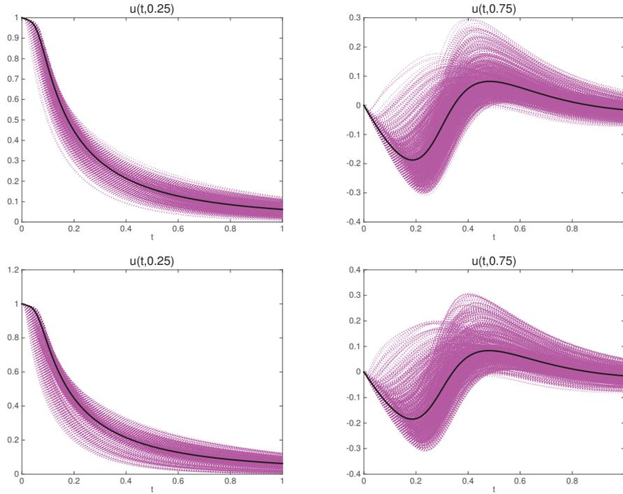
Figure 7: The realisations of the controlled solutions at  $x = 0.25$  (the first column) and  $x = 0.75$  (the second column), which are obtained by the MC method (the first row, 1105 sample points) and the CC grid method with level 5 (the second row, 1105 points). The black lines of all the graphs presents the means of the controlled solutions.
