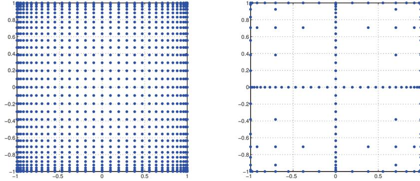
Figure 1: Full tensor product grids using Clenshaw-Curtis abscissas (left). Isotropic Smolyak sparse grids using Clenshaw-Curtis abscissas with level 5 (right).
