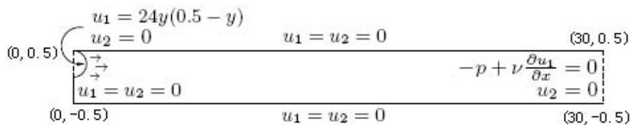
Figure 7: Schematic diagram of the backward-facing step flow.
