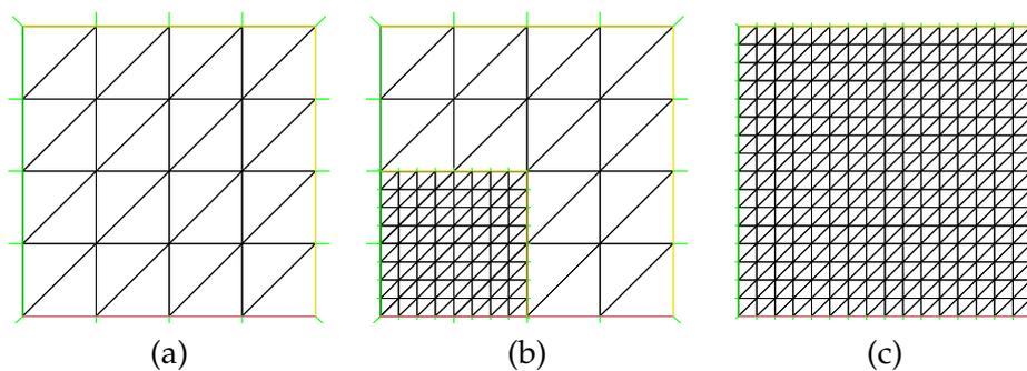
Figure 1: Meshes: (a) a global coarse mesh; (b) a local fine mesh; and (c) a global fine mesh.
