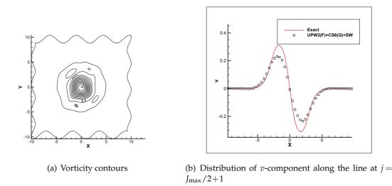
Figure 9: Vorticity contours and v-distributions of UPW3(F)+CS6(G)+SW on  $41 \times 41$  wavy grids in moving vortex problem (Contours from 0 to 0.7 with the number 21).
