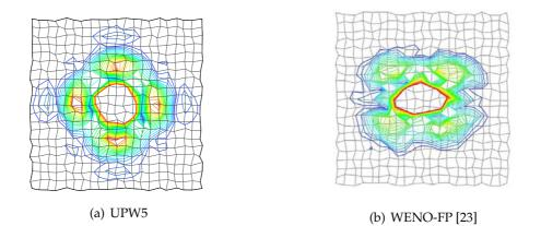
Figure 6: Vorticity contours of different schemes with the courtesy from Ref. [23] (Contours from 0 to 0.005 with number 21).
