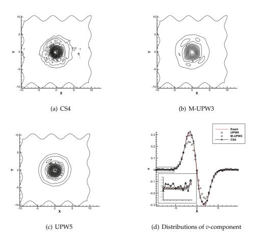
Figure 4: Vorticity contours and v-distributions along the line at  $j=J_{max}/2+1$  on  $41 \times 41$  wavy grids in moving vortex problem (Contours from 0 to 0.7 with the number 21 in (a)-(c)).
