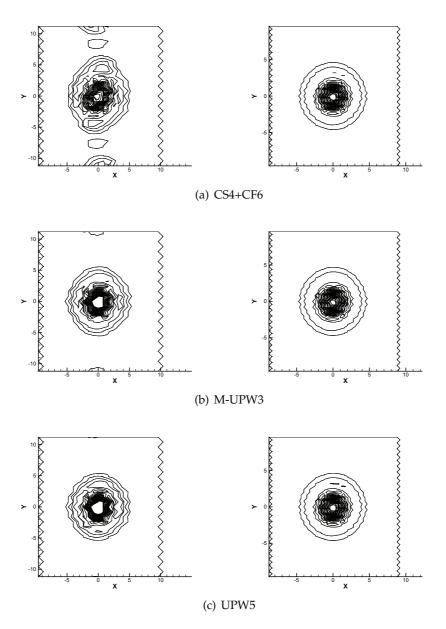
Figure 7: Vorticity contours on  $41 \times 21$  (left) and  $81 \times 41$  (right) triangular-like grids in moving vortex problem (Contours from 0 to 0.7 with number 21).
