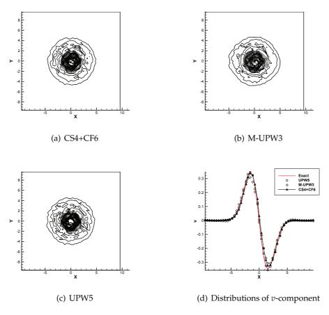
Figure 5: Vorticity contours and v-distributions along the line at  $j = J_{max}/2+1$  on  $41 \times 41$  randomized grids in moving vortex problem (Contours from 0 to 0.7 with the number 21 in (a)-(c)).
