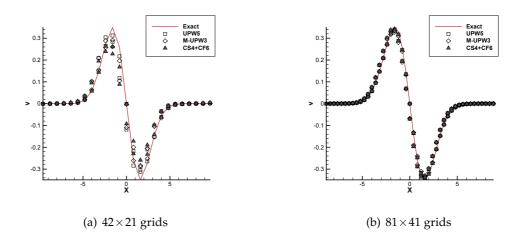
Figure 8: Distributions of v-component along the line at  $j=J_{max}/2+1$  on triangular-like grids in moving vortex problem.
