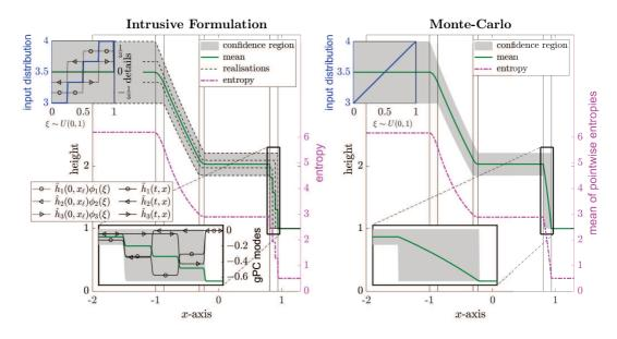
Figure 3: Solution of the dam break problem for the intrusive formulation of Theorem 4.1 compared to a Monte-Carlo simulation in t = 0.5.
