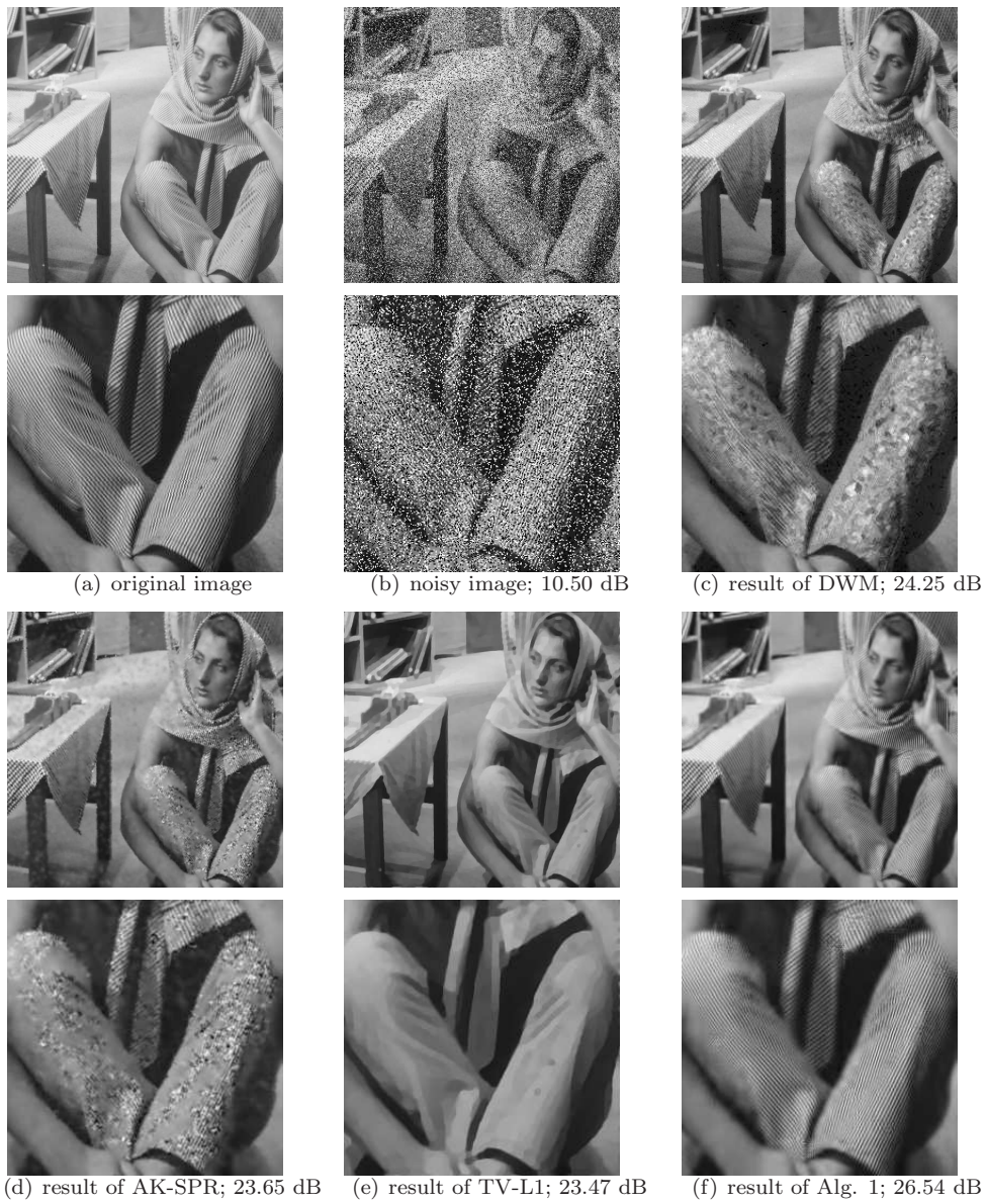
Fig. 5.4. De-noising results for the image “Barbara” corrupted with salt-and-pepper noise.
