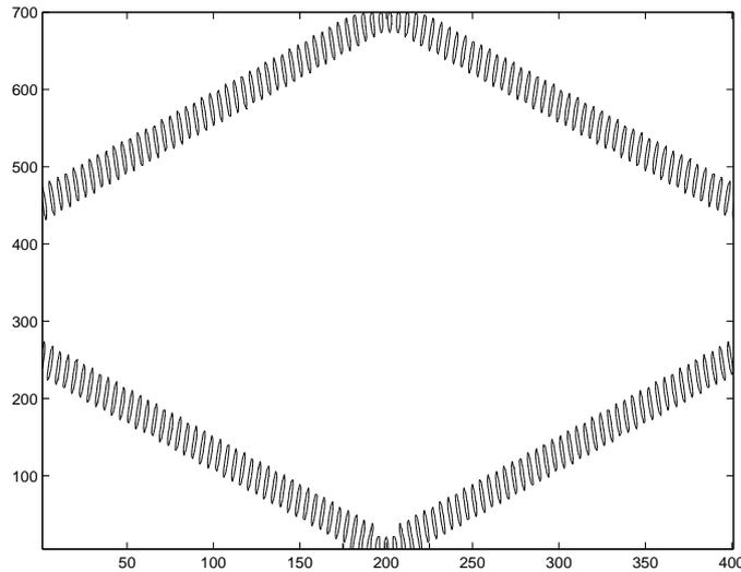
Figure 7: Wave front evolution in the crossing of polychromatic waves. The horizontal axis stands for atomistic numbering  $n$ , and the vertical for time  $t$ .
