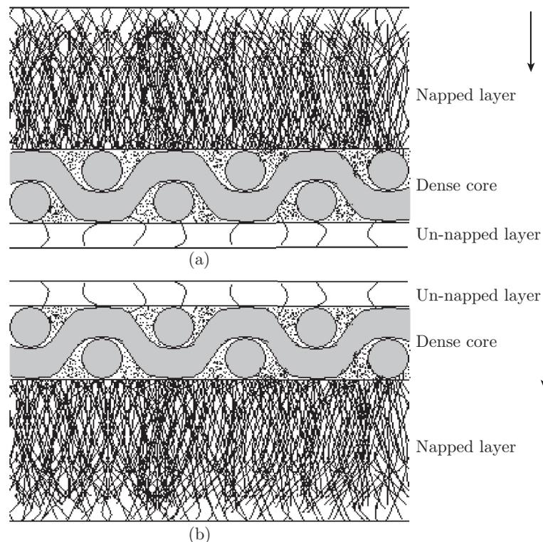
Fig. 12: Schematic diagram of a single-side napped fabric: (a) the upper plate of the FTT contacts the napped layer, (b) the upper plate of FTT contacts the un-napped layer
