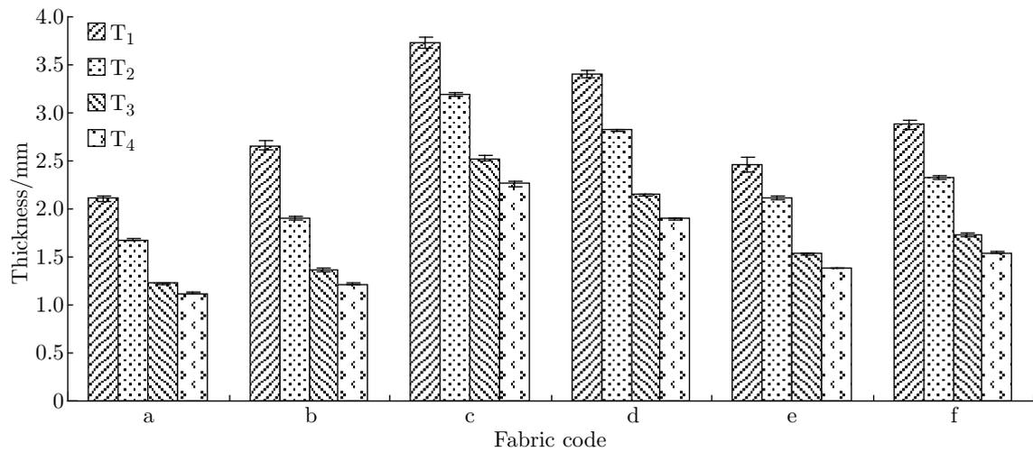
Fig. 8: Thickness of un-napped surface facing upwards at the four measurement points: T<sub>1</sub> represents the initial thickness; T<sub>2</sub> represents the thickness at the first heat peak; T<sub>3</sub> represents the thickness at the standard pressure; T<sub>4</sub> represents the thickness at the max-pressure midpoint
