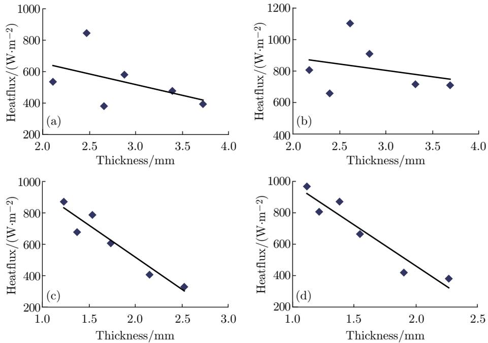
Fig. 10: Linear correlations between the heat flux and thickness for the un-napped surface:  $y$  is the heat flux (W/m<sup>2</sup>) and  $x$  is thickness (mm) at four positions. (a) the initial thickness point  $R^2 = 0.2247$ , (b) the first heat peak point  $R^2 = 0.0762$ , (c) the standard pressure point  $R^2 = 0.9117$ , (d) the midpoint of the maximum pressure  $R^2 = 0.9098$
