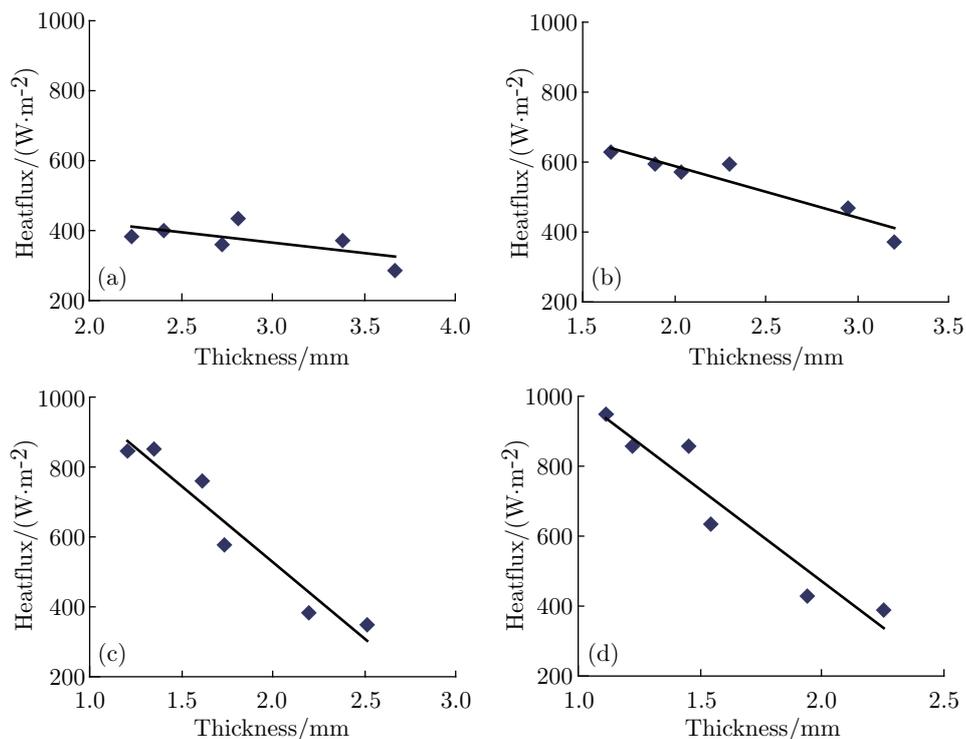
Fig. 11: Linear correlations between the heat flux and thickness for the napped surface: (a) the initial thickness point  $R^2 = 0.4222$ , (b) the first heat peak point  $R^2 = 0.8879$ , (c) the standard pressure point  $R^2 = 0.9315$ ; (d) the midpoint of the maximum pressure  $R^2 = 0.9143$
