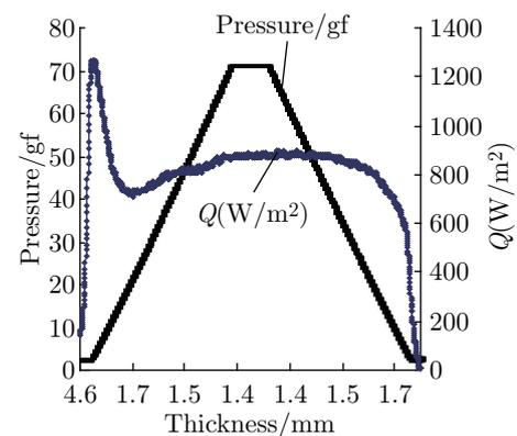
Fig. 4: Curve of pressure and heat flux against thickness for sample e
