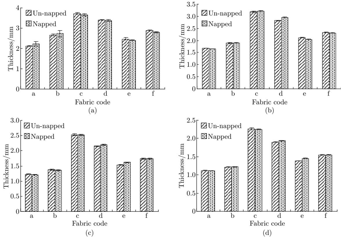
Fig. 7: Comparison of the thickness for the un-napped and napped surfaces: (a) initial thickness, measured surface  $P = 0.928$ ; (b) thickness in the first heat peak, measured surface  $P = 0.750$ ; (c) thickness at standard pressure, measured surface  $P = 0.122$ ; (d) thickness at midpoint of the maximum pressure point, measured surface  $P = 0.065$
