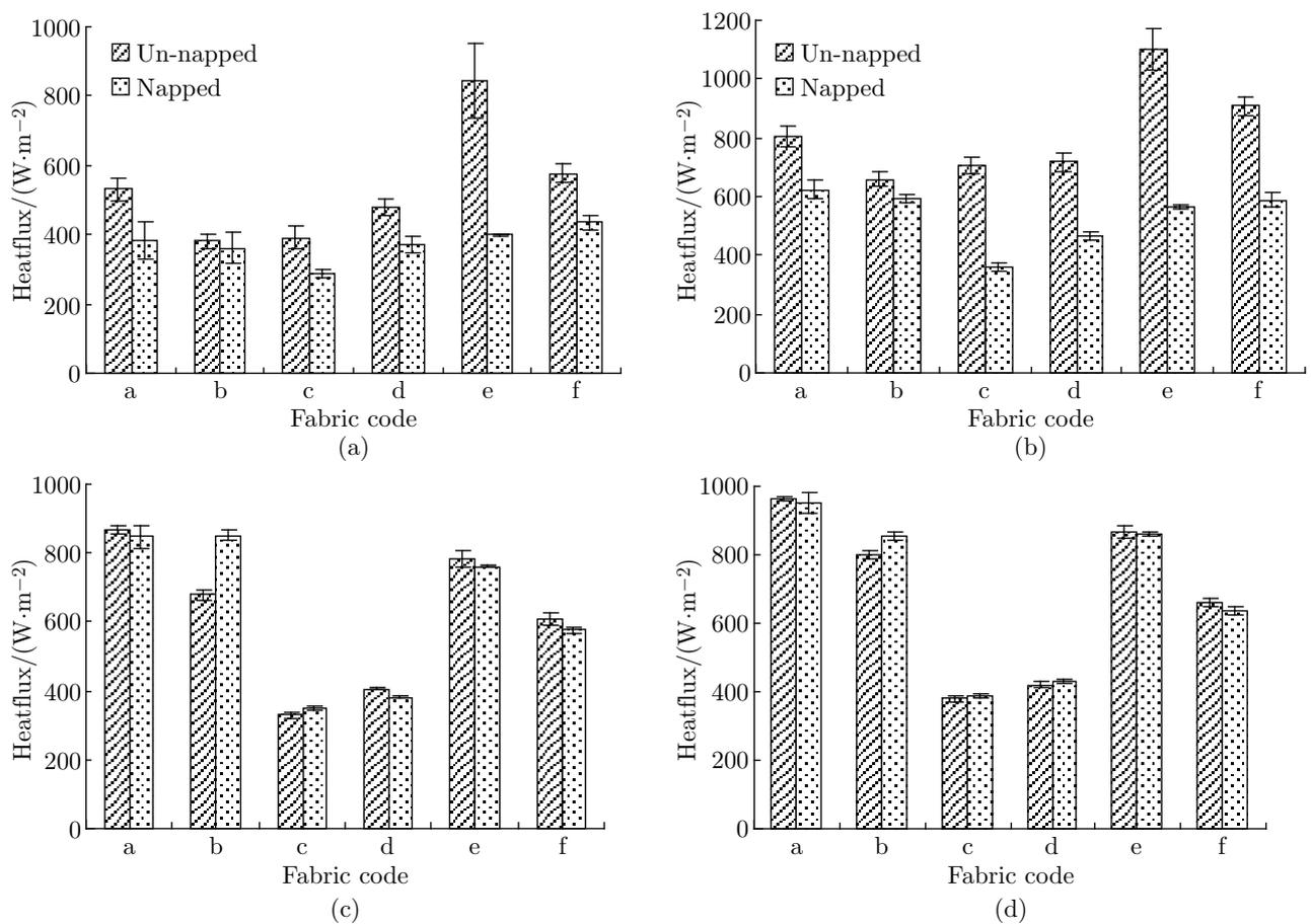
Fig. 9: Comparison of the heat flux for un-napped and napped surfaces: (a) the initial thickness point, measured surface P = 0.000; (b) the first heat peak point, measured surface P = 0.000; (c) the standard pressure point, measured surface P = 0.765; (d) the midpoint of the maximum pressure point, measured surface P = 0.642
