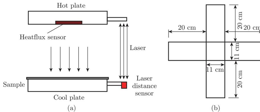
Fig. 1: Measurement principle of the FTT (a) and the dimensions of the cross shape of the sample (b)
