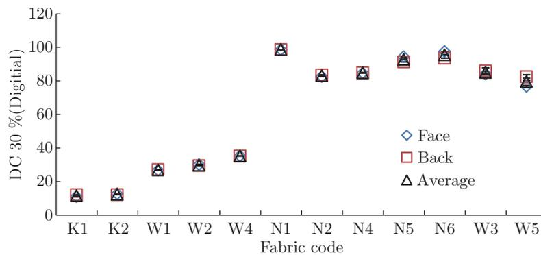
Fig. 6: The drape coefficient measured using 30 cm diameter by the digital method
