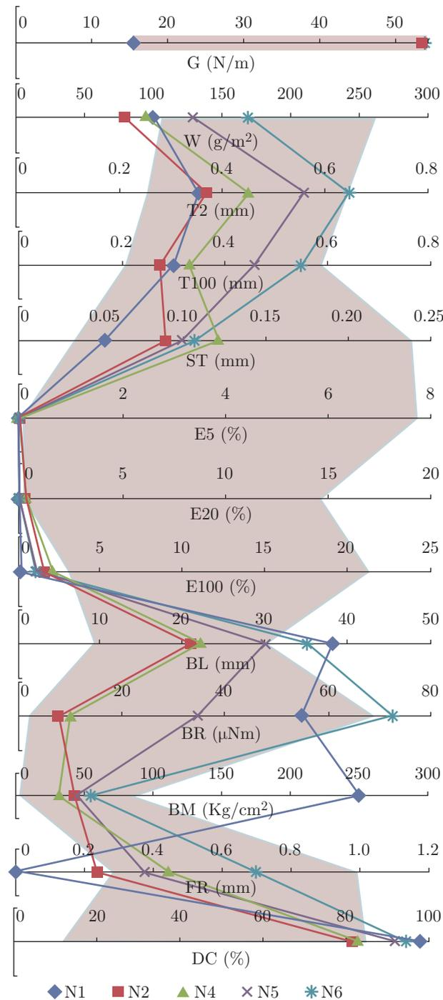
Fig. 7: Correlations between traditional fabrics and nonwovens' measured properties (the shaded areas are for the traditional fabrics)
