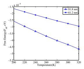
Figure 4: Temperature dependence of the  ${\rm Li}^+$  short-range free energy in LiPON nanoparticles. The particle size in b direction is 100b (61.2 nm) and 150b (91.8 nm).
