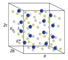
Figure 1: Diffusion channel of Li<sup>+</sup> in LiPON. Blue spheres are interstitial equilibriums  $(I_0)$ . Yellow spheres  $(II_0)$  and gray spheres  $(II^*)$  are metastable sites. a, 2b, and 2c are the sizes along three crystallographic directions.
