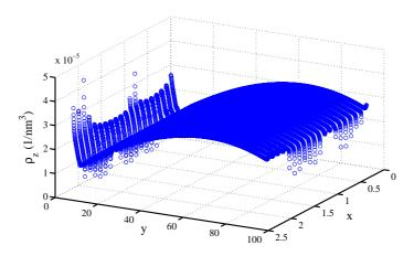
Figure 5:  $Li^+$  ion density in xy plane (z=1.2577 nm).
