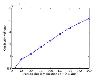
Figure 7: Size effect of the conductivity at 300 K.
