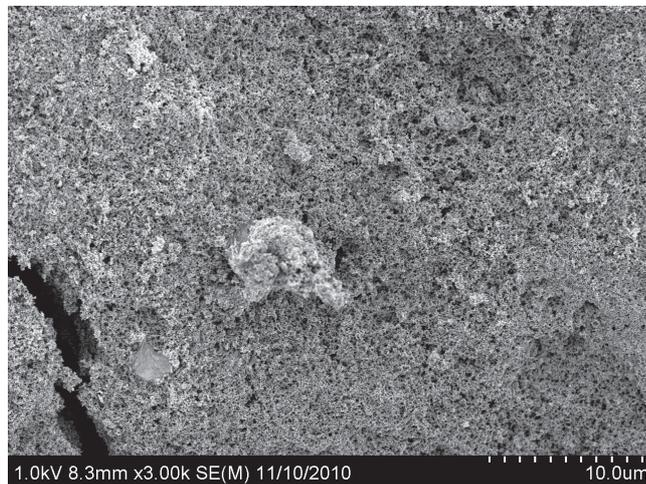
Figure 3: SEM image of the surface of a catalyst layer that has been sprayed onto a membrane.
