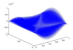
Figure 2: The error between the exact solution  $u_1(x,y) = sin(\pi x)$  and its numerical solution for the  $h = \frac{1}{32}$ .
