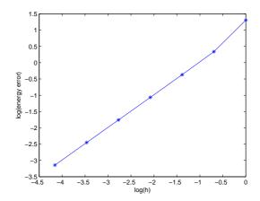
Figure 1: The convergence rate for linear discontinuous finite element.
