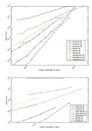
Figure 8: Numerical error in H(div) norm versus the cubic root of number of degrees of freedom for the gaussian source in the cube. Meshes obtained with a deformed pattern (top) and with a split pattern (bottom).
