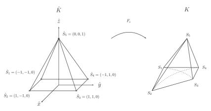
Figure 1: Transformation F for a pyramid.
