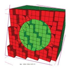
Figure 10: Hybrid mesh used for the sphere.
