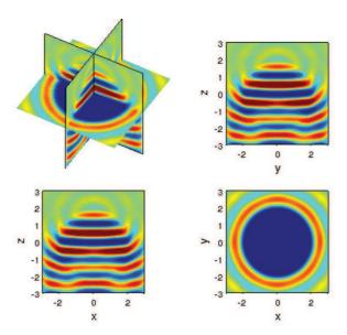
Figure 9: Divergence of u of diffracted field (real part) for the sphere.
