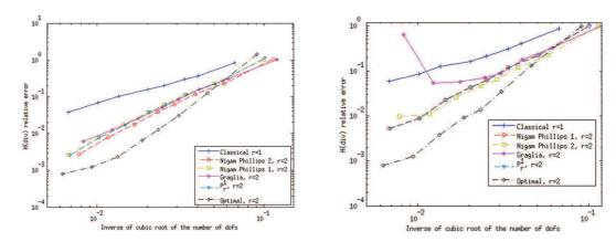
Figure 3: Relative H(div) error for different pyramidal spaces for the source problem with only affine (left) and non-affine (right) pyramids.
