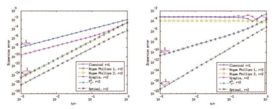
Figure 2: Dispersion error for different pyramidal spaces on a pattern containing only affine (left) and non-affine (right) pyramids.
