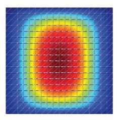
Figure 6: Velocity vectors in x-y plane at z=0.5 (EXAMPLE 4) for scheme (3.11) with h=1/18.
