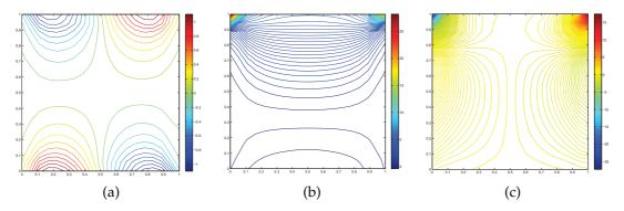
Figure 7: (a)  $\omega_1$  in x-y plane at z=0.5 (EXAMPLE 4); (b)  $\omega_2$  in y-z plane at x=0.5 (EXAMPLE 4); (c)  $\omega_1$  in y-z plane at x=0.5 (EXAMPLE 4), for scheme (3.11) with h=1/18.
