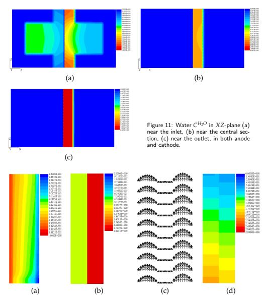
Figure 12: (a) Proton potential  $\Phi_e$  in MEA; (b) Electron potential  $\Phi_s$  in electrode; (c) Velocity field; (d) Pressure field, all in *XY*-plane.
