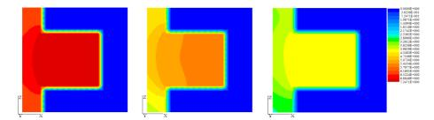
Figure 8: Oxygen  $C^{O_2}$  in XZ-plane (left) near the inlet, (middle) near the central section, (right) near the outlet, in the cathode.
