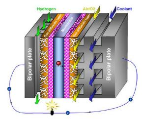
Figure 1: Schematic domain of a 3D PEMFC [62].
