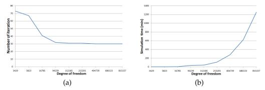
Figure 14: (a) Number of iteration versus degree of freedom; (b) Simulation time versus degree of freedom.
