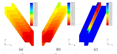
Figure 6: (a) Hydrogen  $C^{H_2}$  in anode; (b) Oxygen  $C^{O_2}$  in cathode; (c) Liquid water saturation s in both anode and cathode.
