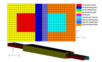
Figure 2: Computational domain and mesh of a single-channel PEMFC.
