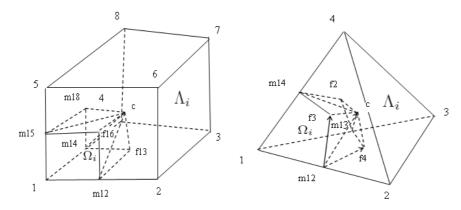
Figure 4: A portion of control volume  $\Omega_i$  surrounded by dotted faces and cell faces in one cell  $\Lambda_i$  of 3D dual mesh.
