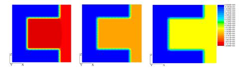
Figure 7: Hydrogen  $C^{H_2}$  in XZ-plane (left) near the inlet, (middle) near the central section, (right) near the outlet, in the anode.
