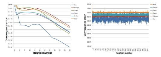
Figure 5: Convergence histories of our FEM-Upwind FVM with Kirchhoff transformation (left) and standard FEM/FVM (right), where the iteration error tolerance is  $10^{-6}$ .
