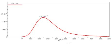
Figure 3: Water diffusivity  $\Gamma(C^{H_2O})$  at 80°C.
