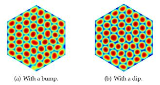
Figure 19: The resulting pattern from a simulation in a hexagonal container with Ma=105, Ra=48, Pr=890, and  $\Gamma=22.0$ . In the left picture we have placed a small bump with a=0.05 and  $\sigma=2.0$  centered at (-5,0). In the right picture we have placed a small dip with a=0.05 and  $\sigma=2.0$  centered at (-5,0). The simulations were started from random initial conditions. The systems evolved into the patterns shown, and remained in this state for about 800 units of dimensionless time.
