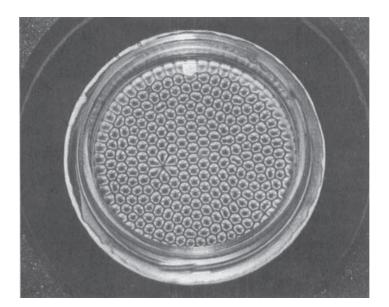
Figure 1: Convection cells (top view) formed due to Bénard-Marangoni convection. We observe cells which are not hexagonal in nature and which locally form a star-like pattern (a dislocation). The experimental result is taken from [21] and is reprinted here with permission from Wiley.
