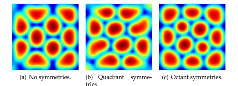
Figure 12: Resulting patterns from simulations where we enforce (a) none, (b) quadrant, or (c) octant symmetries on the initial conditions for the temperature. The final patterns are quite different, an indication that we are able to influence the pattern selection process through our choice of initial condition.
