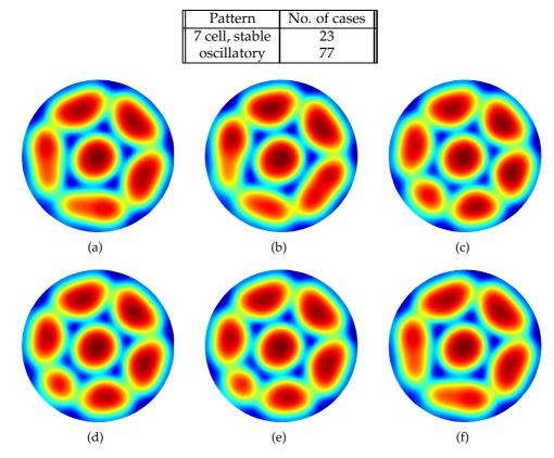
Figure 15: Final oscillatory pattern after long time integration in a circular container with Ma = 105, Ra = 48, Pr = 890 and  $\Gamma = 8.38$ . The plots show 6 evenly spaced snapshots over a single period. There is a small bump with a = 0.05,  $\sigma = 0.2$  centered at (-2, -2). This results in a steady periodic flow pattern.
