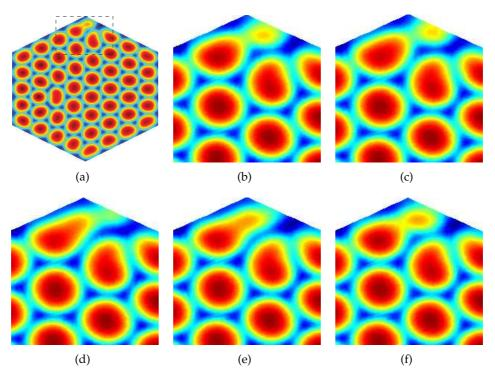
Figure 9: Final oscillatory pattern after long time integration for a hexagonal container with Ma=105, Ra=48, Pr=890, and  $\Gamma=22$ . The overall pattern is shown in (a), while the remaining plots show a close-up of the pattern near the oscillatory cell at different times during one period.
