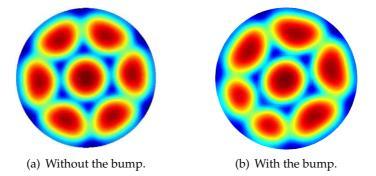
Figure 16: The resulting pattern from two computations. The left figure shows the resulting pattern in the container without the bump. The right figure shows the stationary pattern obtained when there is a bump at the bottom. The right pattern resembles the left one, except locally where the bump is placed, the system behaves as if the fluid layer is thinner.
