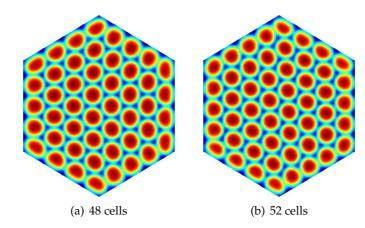
Figure 8: Two different resulting flow patterns in a hexagonal container with Ma = 105, Ra = 48, Pr = 890, and  $\Gamma = 22$ . The only difference between the two simulations is the random initial condition for the temperature. The 48-cell configuration appears to be the most common, while the 52-cell configuration is a more exceptional case.
