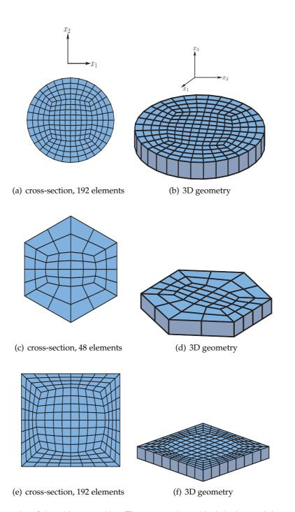
Figure 2: Some examples of the grids we consider. The cross-sections with their elemental decomposition are given in the left column. As can be seen in the right column, we here only consider a single layer of spectral elements in the vertical direction.
