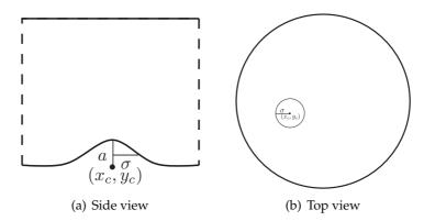
Figure 14: A cylindrical container with a Gaussian bump at the bottom. (a) Side view of the bump centered at  $(x_c, y_c)$  with standard deviation  $\sigma$ . We have here zoomed in on the bump to highlight the definition of the parameters. b) Top view showing a sample placement of the bump.
