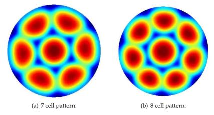
Figure 7: Two possible cell patterns obtained at steady state for Ma = 105, Ra = 48, Pr = 890, and  $\Gamma = 8.38$ .
