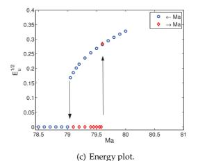
Figure 4: A plot of the energy measure  $E_u^{1/2}$  at steady state for different values of the Marangoni number. Our estimate of the critical Marangoni number is 79.6, while the subcritical regime extends down to Ma=79.1. The obtained values are in good agreement with previously reported results [9, 36, 39].
