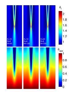
Figure 5: Convergence study, using same setup as case A = 0.2 in Fig. 4. From left to right, we use resolutions of (K=10,M=60), (K=10,M=120), and (K=20,M=320). The DG order is taken as N=6. In the coarsest resolution we see numerical oscillations in the melt channels; these disappear with refinement.
