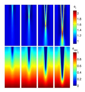
Figure 4: Steady-state solutions with sustained inflow porosity perturbation as given in (5.1). Top: fluid fraction. Bottom: opx abundance. From left to right, perturbation amplitude  $A = \{0.05, 0.1, 0.2, 0.4\}$ .
