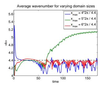
Figure 7: Expected wavenumber  $\langle k \rangle$  as a function of time for varying horizontal domain length  $x_{max}$ . The assumption of periodic boundary conditions constrains which wavenumbers we are able to represent.
