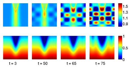
Figure 6: Evolution of fluid fraction (top) and opx abundance (bottom) in unstable wave regime with fixed boundary perturbation (5.1). Interaction between porosity waves, inherent to the system, and a central channel, induced by the boundary condition, is observed. Outflow dunite (opx-free) channels are shown to vary in time as strong porosity waves emerge.
