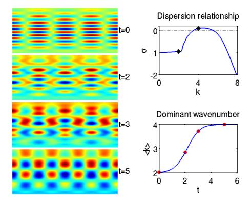
Figure 3: Wavenumber selection. Initially most of the energy is focused in the stable k=2 mode, with a small amount in the unstable k=4 mode. As predicted by linear stability analysis, the former decays while the latter emerges as the dominant feature.
