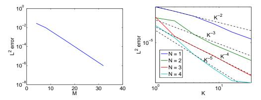
Figure 1: Convergence study.  $L^2$  error rates in porosity  $\phi_f$  are shown. The error decays exponentially as a function of FC order M and DG order N, and polynomially as a function of element size  $K^{-1}$ . Dashed black lines in right panel denote reference lines of slope  $K^{-(N+1)}$ .
