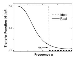
Figure 3: Transfer function for eliminating reflected phonons.  $\omega_t$  is the minimum frequency of total reflection. The dashed line is the ideal transfer function. The solid line is a realistic transfer function we obtained for a one dimensional system as described by Eq. (2.10).
