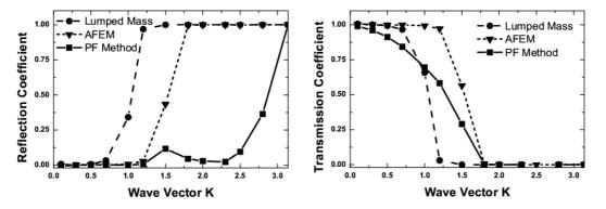
Figure 5: A comparison of reflection and transmission coefficients using numerical simulations. The  $\blacksquare$  line,  $\blacktriangle$  line and  $\bullet$  line are the result of AFEM with PF method, AFEM and lumped mass FE method, respectively.
