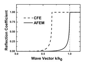
Figure 2: Comparison of the calculated reflection coefficient for AFEM and conventional FE methods with lumped mass approximation. The AFEM can largely improve the transparency.
