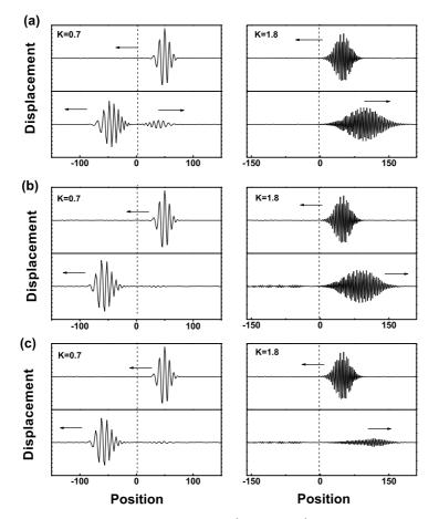
Figure 4: Gaussian wave packet of small wave vector (left column) and large wave vector (right column) travelling from the MD region to FE region. (a) lumped mass FE method; (b) AFEM; (c) AFEM with PF method. The dashed line denotes the atomistic/continuum interface. It is clear that PF has little effect on the small wave vector packet, while it dampens the large wave vector packet.
