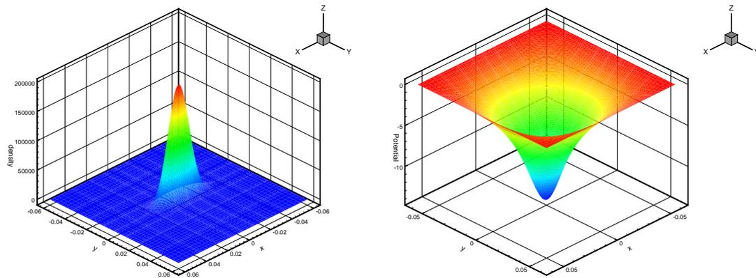
Figure 15: Charge density in physical space  $(x,y)$  (left); Electric potential distribution obtained by solving 2D Poisson's equation (right).
