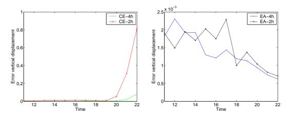
Figure 9: Evolution of the error along the z=0 surface for  $11 \le t \le 22$ , for the Clayton-Engquist (left) and the energy absorbing (right) far field boundary conditions. Here,  $c_p/c_s=10$  and the two curves correspond to h=0.02 and h=0.04, respectively. Note that the vertical scale goes from 0 to 1 in the left plot, but from 0 to  $2.5 \times 10^{-3}$  in the right plot.
