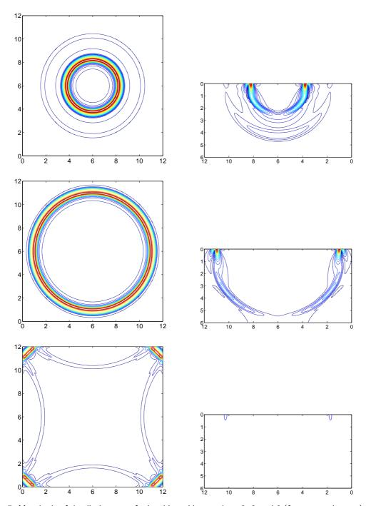
Figure 7: Magnitude of the displacement for Lamb's problem at times 3, 6, and 9 (from top to bottom) in the z=0 plane (left) and y=6 plane (right). The energy absorbing far-field boundary condition (3.16) was used to truncate the computational domain in this calculation, which used the grid size h=0.02. The contour levels are the same in all plots and are equally spaced between 0 and 0.15 with interval 0.00375.
