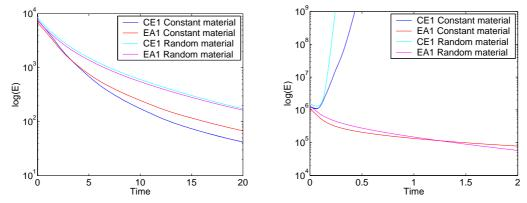
Figure 4: Logarithm of energy vs. time when  $c_p/c_s = 1.732$  (left) and when  $c_p/c_s = 30$  (right). Random initial data. Constant material (blue and red curves) and randomly varying material (cyan and magenta curves).
