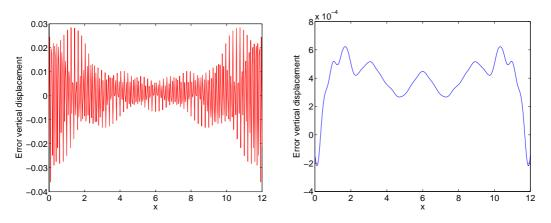
Figure 10: The error along the line z=0, y=6 at t=22, for the Clayton-Engquist (left) and the energy absorbing (right) far field boundary conditions. Here,  $c_p/c_s = 10$  and h = 0.04. Note that the vertical scale goes from -0.04 to 0.03 in the left plot, but from  $-4 \times 10^{-4}$  to  $8 \times 10^{-4}$  in the right plot.
