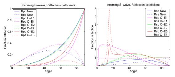
Figure 3: Reflection coefficients when  $c_p/c_s = 30$ . Incident *P*-wave (left) and incident *S*-wave (right). Solid curves are *P* wave reflections and dashed curves are *S* wave reflections.
