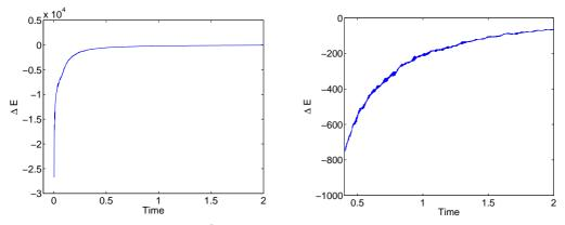
Figure 5: Energy difference  $\Delta E(t_n) = E^{n+1} - E^n$  as function of time when  $c_p/c_s = 30$  for the energy absorbing boundary condition. A closeup for later times is shown in the right subfigure. Note that the scale on the vertical axis goes from  $-3 \times 10^4$  to  $5 \times 10^3$  in the left subplot, and from -1000 to 0 in the right subplot.
