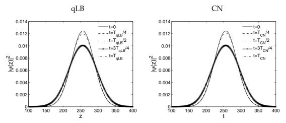
Figure 5: Wave function densities computed by qLB and CN. Parameters are set as follows:  $N_z = 512$ ,  $z_0 = 256$ ,  $\tilde{m} = 1/4$ ,  $\Delta_0 = 32$ ,  $\omega_0 = 1/512$ ,  $v_z = 0.0$ ,  $V_{nl} = 0.1$ . For qLB  $|\psi(z,t)|^2$  is computed at times 0,  $T_{qLB}/4$ ,  $T_{rcN}/4$ ,  $T_{CN}/2$ ,  $3T_{CN}/4$  and  $T_{CN}$ .
