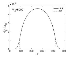
Figure 12: Ground state profile  $\phi_g(z,y)$  taken at  $y=y_0$  for different values of  $V_{nl}$  and compared with the Thomas-Fermi wave function (see Eq. (8.9)). Simulation parameters are set as:  $\tilde{m}=1/8$ ,  $\Delta_{0z}=\Delta_{0y}=16$ ,  $\omega_0=1/128$ ,  $N_z=N_y=512$ . Solid lines: qLB model; dashed lines: Thomas-Fermi approximation. Space is expressed in lattice units. The tails associated with the kinetic energy contribution are well visible.
