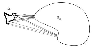
Figure 19: Interaction in one iteration between the subscatterers for the element at  $x_i$  on  $\Omega_1$ . The element is assumed to radiate as a point source. Rays bouncing off  $\Omega_2$  and hitting the elements on  $\Omega_1$  are shown. Note that for some elements on  $\Omega_1$  there are multiple returning rays.
