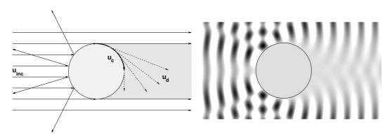
Figure 4: Diffraction by a smooth cylinder. Left figure shows the solution schematically. The incident field  $u_{\rm inc}$  induces a creeping ray  $u_{\rm c}$  at the north (and south) pole of the cylinder. As the creeping ray propagates along the surface, it continuously emits surface-diffracted rays  $u_{\rm d}$  with exponentially decreasing initial amplitude. Right figure shows the real of a solution to the Helmholtz equation. The surface diffracted waves can be seen behind the cylinder.
