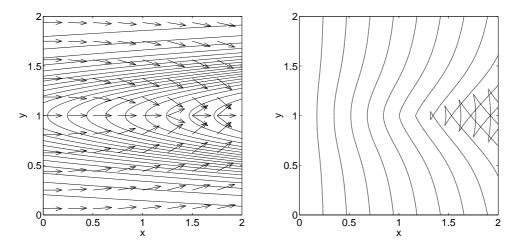
Figure 15: Results for the lens simulation. Left frame: local ray directions with contour lines of index of refraction overlayed; right frame: wave front in the xy-plane for a sequence of arrival times (T-values).
