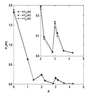
Figure 8: A typical magnetic moment on the Cu site as a function of  $V_{pd}$  and doping concentration [59].
