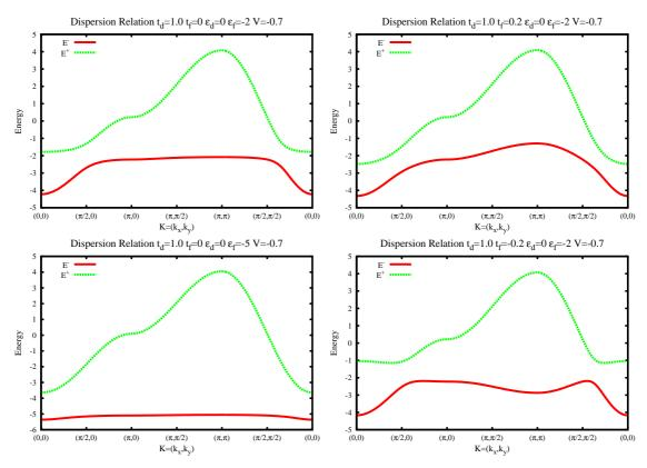
Figure 6: Dispersion of the periodic Anderson model (a) for the case of zero  $t_f$ , (b) for the case of positive  $t_f$  (c) for the case of zero  $t_f$  with a large band gap, (d) for the case of negative  $t_f$
