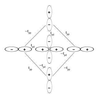
Figure 4: Phase convention for the hopping matrix elements. The copper  $d_{x^2-y^2}$  orbital is surrounded by the oxygen  $p_x$  and  $p_y$  orbitals. The hopping matrix elements are shown with their corresponding phase.
