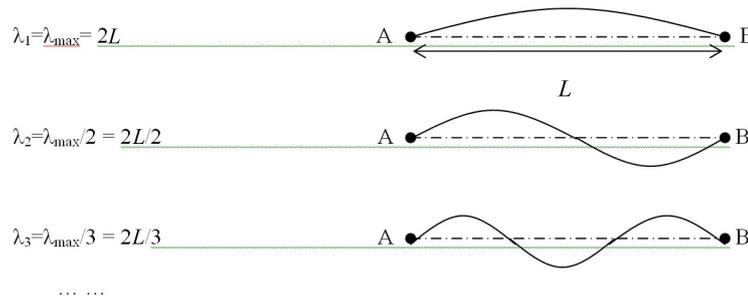
Figure 2: Schematic of the stable stationary wave modes ( $L$ , the distance)
