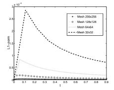
Fig. 4.4. Comparison of the evolution of  $L_1$ -norm at different meshes and N = 10.
