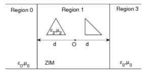
Figure 1: The schematic description of the waveguide structure with vacuum (regions 0 and 3), ZIM (region 1), and embedded triangular defects.
