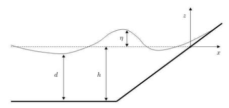
Figure 1: The reference frame of the DNSWE.
