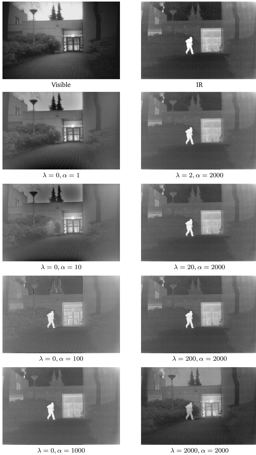
Figure 9: A visible image, an infrared image and the fused images by our model and ALM-FFTs with different parameters \lambda and \alpha .
