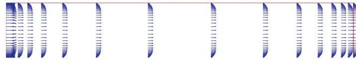
Figure 4: Velocity field of developing supercritical CO 2 flow in the Channel at Re_{in}=210 and q=400 .
