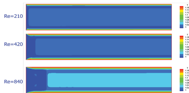
Figure 10: Distributions of temperature inside the channel at three Reynolds numbers and q=800 [W/m].
