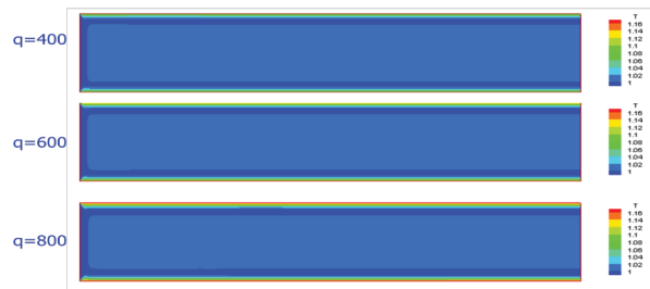
Figure 9: Distributions of temperature inside the channel at Re_{in}=210 and heat flux boundary conditions.
