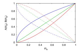
Figure 1: (Color online) Linear (green), retarded (red) and advanced (blue) annealing schemes for qubit *i*. The dashed lines indicate  $A_i(t/t_a) = 1 - (t/t_a)^{1+\gamma_i}$  with  $\gamma_i = -0.5$ , 0, and 0.5 (bottom to top). The solid lines indicate  $B_i(t/t_a) = (t/t_a)^{1+\gamma_i}$  with  $\gamma_i = -0.5$ , 0, and 0.5 (bottom).
