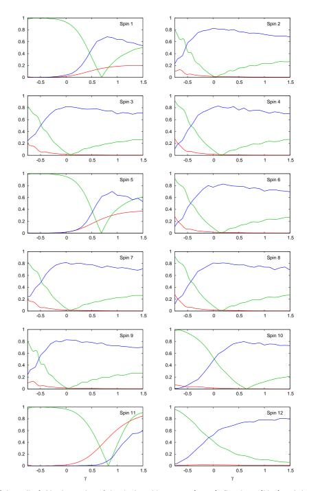
Figure 2: (Color online) Absolute value of the single-qubit average (green), floppiness (blue) and the probability for finding the ground state (red) as a function of the anneal offset  $\gamma$  for each spin in the 12-spin 2-SAT problem with number 487.
