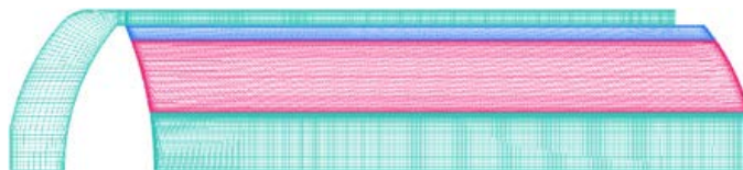
Figure 3: Schematic diagram of axisymmetric mesh of vertical radial flow adsorber.
