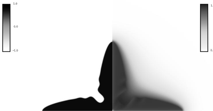
Figure 2: The 2-d interface shape at time  $t = 1800$ , showing the phase solution on the left, and the solute profile on the right.
