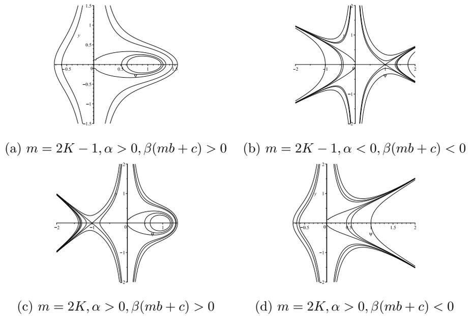
**Figure 2.** The bifurcation phase portraits of the system (3.1) for  $n = 2, A = 0, K = 1, 2, \dots$
