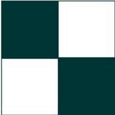
Figure 3: Jumps in Young's modulus, namely  $E=E_1$  on dark subdomains and  $E=E_2=10^3$  on light ones.
