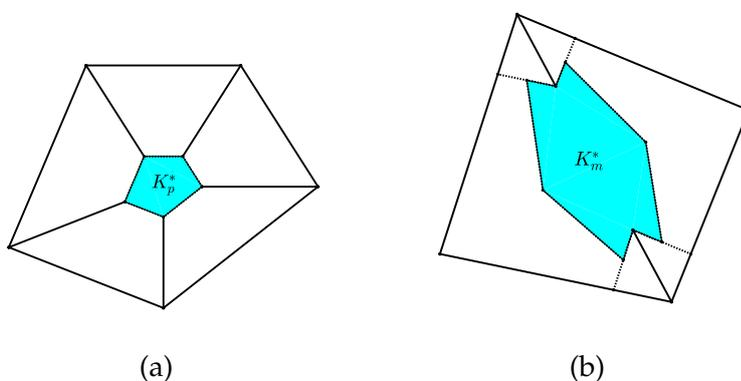
Figure 2: (a): Control volume around a vertex, (b): Control volume around a midpoint.
