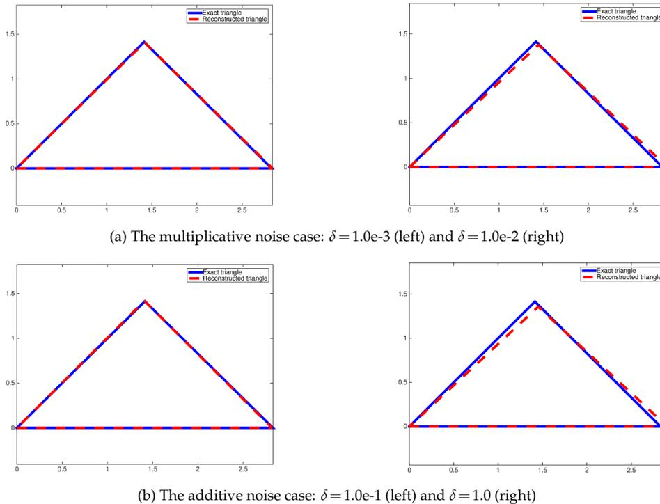
Figure 3: The comparisons of the exact and reconstructed triangles for Example 3.1 with noisy eigenvalues.
