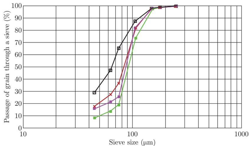
Fig. 2: Distribution curve of the characteristic opening size of needle punched polypropylene sample with  $450 \text{ g/m}^2$
