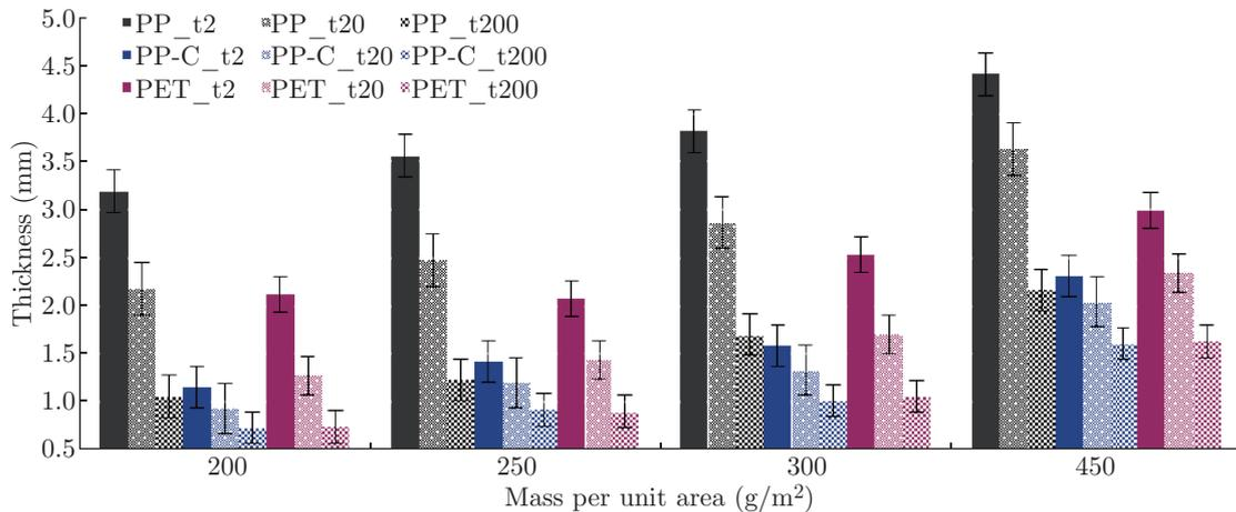
Fig. 3: Change of thickness on nonwoven geotextiles caused by applied pressures in dependence of mass per unit area with associated standard error bars
