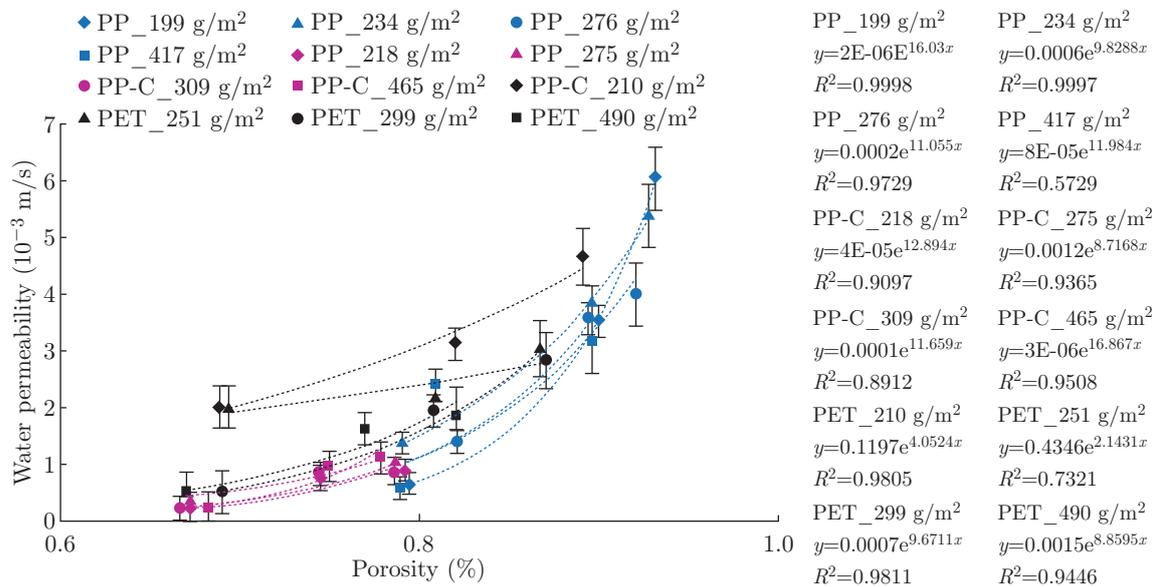
Fig. 9: Dependence of water permeability under applied pressures and porosity of nonwoven geotextiles
