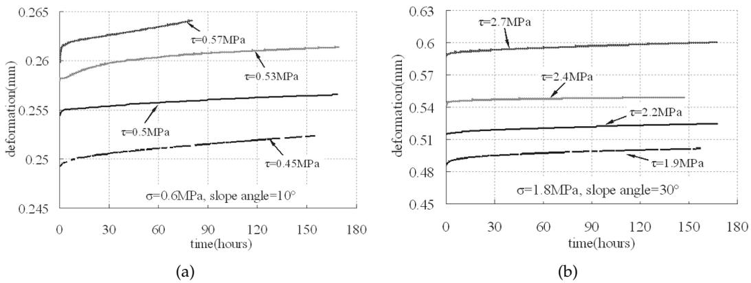
Figure 3: The grading curves of shear creep of 10° and 30° structural planes.
