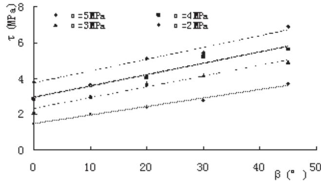
Figure 1: The relationship between peak shear strength and discontinuity angle.
