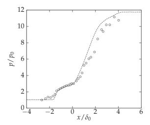
Figure 12: Compression corner M=5, Flow Case 6. Experimental values from Dolling *et al.* [10]. Results obtained on a grid with size:  $384 \times 160$ .
