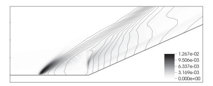
Figure 7: Flow Case 2  $\alpha$  = 24°. Degree of rarefaction according to Eq. (2.49) in supersonic compression corner flow, M = 2.85 (iso-contours in grayscale). 20 pressure contour lines have been added for reference.
