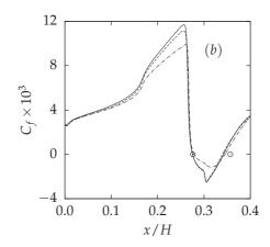
Figure 1: Pressure (a) and skin friction coefficient (b) for the Délery bump channel flow. (———) Gas-kinetic scheme (GKS) on finest grid, (–––––) GKS on medium grid, (–––––) GKS on coarsest grid, (—–—) Navier-Stokes (Roe's approximate Riemann solver) on finest grid, (  $\sigma$  ): experimental data from Délery [8]. Size of coarse, medium and fine grids:  $200 \times 160$ ,  $312 \times 256$ ,  $456 \times 288$  respectively.
