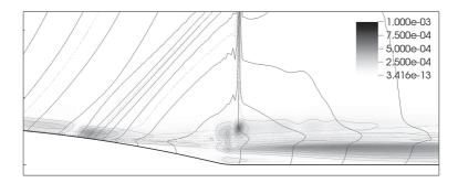
Figure 2: Degree of rarefaction according to Eq. (2.49) (iso-contours in grayscale) for Délery bump channel flow. 20 pressure isocurves have been added for reference.
