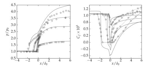
Figure 6: Flow Case 2. Pressure and friction coefficient calculated for four different compression corner flows, with angles of  $8^{\circ}$ ,  $16^{\circ}$ ,  $20^{\circ}$  and  $24^{\circ}$  (freestream conditions: M=2.85,  $Re=7.0\times10^{7}$  per length unit,  $\delta_0=0.023m$ ). (———) GKS on finest grid, ( o ): experimental data from Settles [26].
