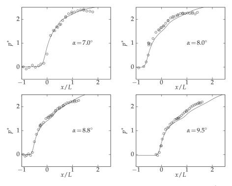
Figure 10: Flow Case 5. Reflected shock wave at low Reynolds number and Mach  $M\!=\!2.3$  (experimental data from [11]) with angles ranging from 7.0 to 9.5 degrees.  $p^*\!=\!(p\!-\!p_1)/(p_2\!-\!p_1)$ , where  $p_1$  and  $p_2$  are the inviscid pressure values upstream and downstream of shock, respectively. The interaction length L is measured from the foot of the reflected shock to the reattachment point. Results obtained on a grid with size:  $496\!\times\!304$ .
