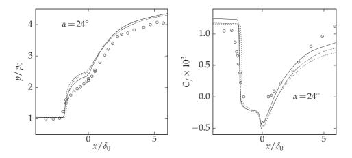
Figure 5: Flow Case 2. Grid convergence. (freestream conditions: M=2.85,  $Re=7.0\times10^7$  per length unit,  $\delta_0=0.023m$ ). (———) Gas-kinetic scheme (GKS) on finest grid, (----) GKS on medium grid (only shown for  $\alpha=24^\circ$ ), (-----) GKS on coarsest grid (only shown for  $\alpha=24^\circ$ ), (o): experimental data from Settles [26].
