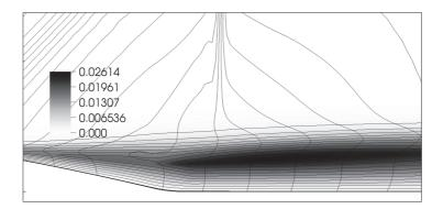
Figure 4: Flow Case 1. Non-dimensional  $\tau_{xy}$  component of the turbulent stress tensor in Délery bump channel flow. Experimental values can for instance be found in the measurements by Sartor *et al.* [25].
