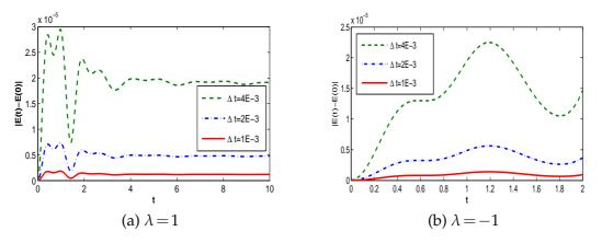
Figure 1: Energy error of TSFP in defocusing case ( $\lambda = 1$ ) and focusing case ( $\lambda = -1$ ): |E(t) - E(0)| for different  $\Delta t$  during the computing under  $\Delta x = 1/8$  and  $\varepsilon = 1$ .
