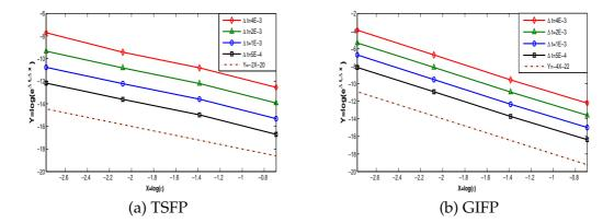
Figure 2: Dependence of the temporal discretization error on  $\varepsilon$  (in log-scale) for different  $\Delta t$  at t=1 under  $\Delta x=1/8$ : (a) for TSFP and (b) for GIFP.
