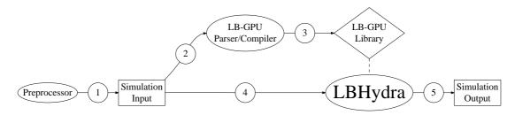
Figure 2: LBHydra GPU simulation pipeline. The preprocessor generates an input file (1) which is first read (2) by the Parser/Compiler to generate (3) a dynamic library linked to the main LBHydra program. The input file is then read (4) by LBHydra which uses the newly-created library to run the GPU simulation (5).
