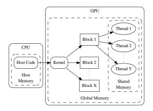
Figure 1: GPU kernel execution is based on groups of threads known as thread blocks. Inter-thread communication is made possible through shared memory, accessible to all threads within the same block. In addition, threads have access to the GPU's global memory, a larger data storage space which is available on the device, distinct from the CPU host's memory.
