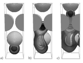
Figure 3: LBHydra's GPU module models a buoyant droplet of CO<sub>2</sub> dissolving in ambient water within a regular array of spheres. Contour surfaces indicate concentrations of dissolved CO<sub>2</sub> between 5% and 95% of the saturation concentration. The innermost contour denotes the surface of the pure CO<sub>2</sub> droplet. Lattice dimensions:  $100 \times 100 \times 300$ .
