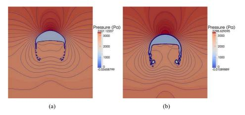
Figure 15: Comparison of the computed bubble shapes at t = 5.4s, contoured by pressure. (a) final bubble shape computed by current proposed model; (b) final bubble shape computed by the single phase explicit model reported in [10].
