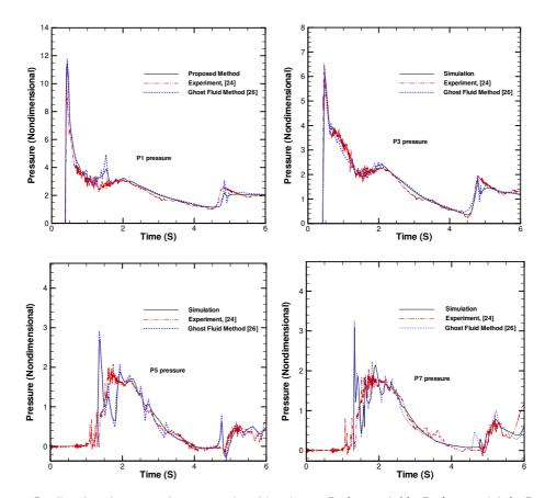
Figure 11: Predicted and measured pressure time histories at  $P_1$  (upper left),  $P_3$  (upper right),  $P_5$  (bottom left) and  $P_7$  (bottom right). Results by GFM (see [26]) are also presented for comparison. The pressure was nondimensionalized by dividing  $\rho_{ref}U_{max}^2$ , where  $\rho_{ref}$  is the density of water and  $U_{max}$  the maximum velocity in the field.
