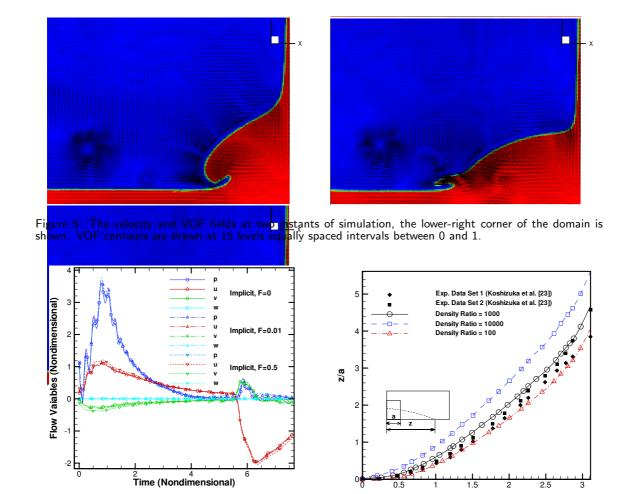
Figure 6: The comparisons of solution accuracy by setting different values of deactivation interface position (F=0, F=0.01 and F=0.5). The grid with 140×80×4 points were used. GMRES+ILU employed.
