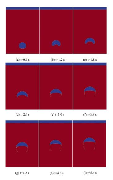
Figure 14: Time evolution of the single rising bubble. The bubble shape is contoured by VOF number F = 0.5.
