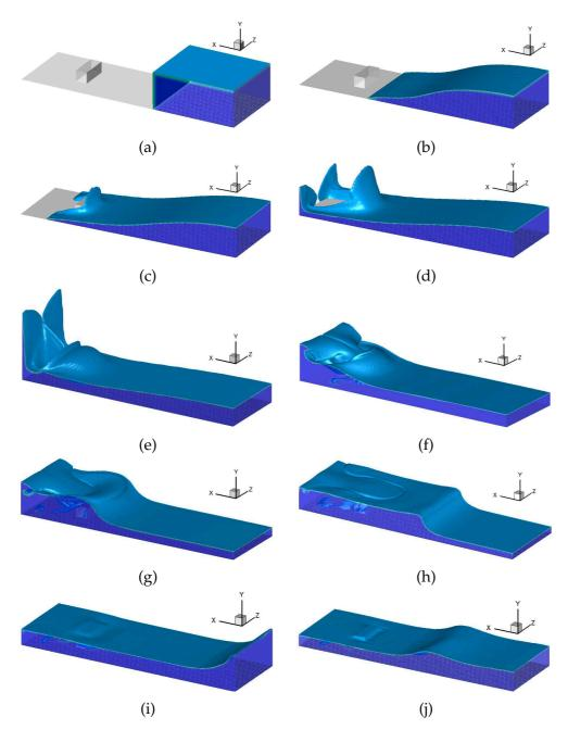
Figure 9: Snapshots of predicted dam breaking wave interacting with obstacle in early stages. ISO surface by F=0.5. Implicit scheme, GMRES+ILU on mesh with 1,008,857 grid points and 5,882,357 tetrahedral elements.
