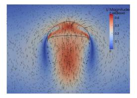
Figure 16: Instant shape of the single rising bubble at t = 5.4s, contoured by VOF number F = 0.5. Figure is colored by velocity magnitude. Velocity vectors are also plotted.
