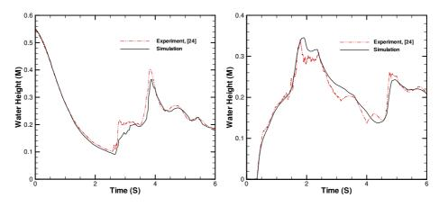
Figure 10: Predicted water depth in the reservoir  $H_4$  (left) and the tank  $H_2$  (right).
