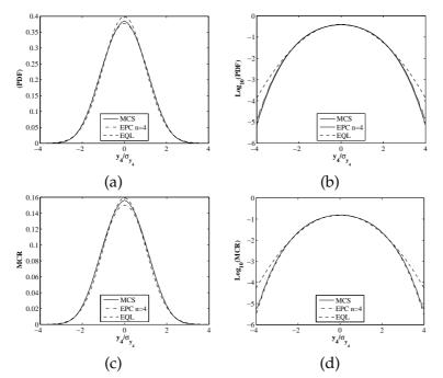
Figure 12: Comparison of PDFs, logarithmic PDFs, MCRs, and logarithmic MCRs in example 4: (a) PDFs of displacement  $Y_4$ ; (b) Logarithmic PDFs of displacement  $Y_4$ ; (c) MCRs at  $Y_4 = y_4$ ; (d) Logarithmic MCRs at  $Y_4 = y_4$ .
