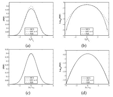
Figure 3: Comparison of the PDFs and logarithmic PDFs in example 1: (a) PDFs of displacement  $Y_5$ ; (b) Logarithmic PDFs of displacement  $Y_5$ ; (c) PDFs of velocity  $\dot{Y}_5$ ; (d) Logarithmic PDFs of velocity  $\dot{Y}_5$ .
