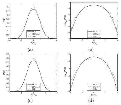
Figure 8: Comparison of the PDFs and logarithmic PDFs in example 3: (a) PDFs of displacement  $Y_3$ ; (b) Logarithmic PDFs of displacement  $Y_3$ ; (c) PDFs of velocity  $\dot{Y}_3$ ; (d) Logarithmic PDFs of velocity  $\dot{Y}_3$ .
