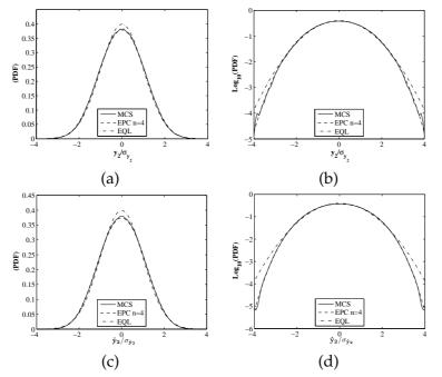
Figure 4: Comparison of the PDFs and logarithmic PDFs in example 2: (a) PDFs of displacement  $Y_2$ ; (b) Logarithmic PDFs of displacement  $Y_2$ ; (c) PDFs of velocity  $\dot{Y}_2$ ; (d) Logarithmic PDFs of velocity  $\dot{Y}_2$ .
