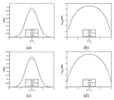
Figure 7: Comparison of the PDFs and logarithmic PDFs in example 3: (a) PDFs of displacement  $Y_2$ ; (b) Logarithmic PDFs of displacement  $Y_2$ ; (c) PDFs of velocity  $\dot{Y}_2$ ; (d) Logarithmic PDFs of velocity  $\dot{Y}_2$ .
