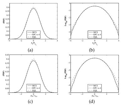
Figure 5: Comparison of the PDFs and logarithmic PDFs in example 2: (a) PDFs of displacement  $Y_3$ ; (b) Logarithmic PDFs of displacement  $Y_3$ ; (c) PDFs of velocity  $\dot{Y}_3$ ; (d) Logarithmic PDFs of velocity  $\dot{Y}_3$ .
