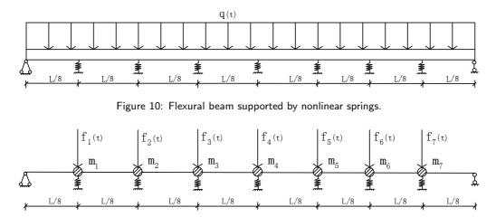
Figure 11: Model for dynamic analysis of the flexural beam.
