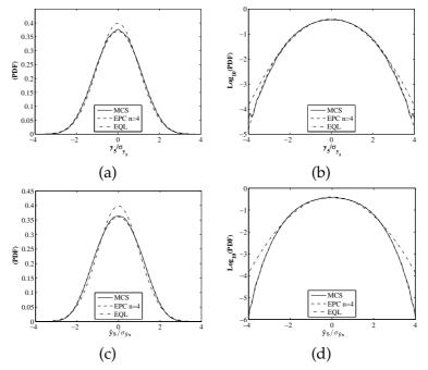
Figure 6: Comparison of the PDFs and logarithmic PDFs in example 2: (a) PDFs of displacement  $Y_5$ ; (b) Logarithmic PDFs of displacement  $Y_5$ ; (c) PDFs of velocity  $\dot{Y}_5$ ; (d) Logarithmic PDFs of velocity  $\dot{Y}_5$ .
