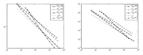
Figure 23: Example 5.5: the  $H^1$  (left) and  $L^2$  (right) error against the #DOF with comparison of linear and quadratic approximation using the ZZ error estimator.
