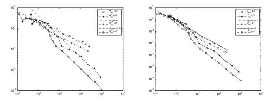
Figure 11: Example 5.1: the  $H^1$  (left) and  $L^2$  (right) error against the #DOF with comparison of quadratic and linear interpolation of f.
