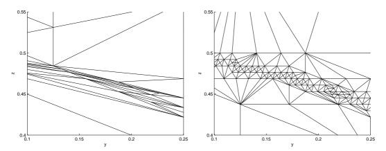
Figure 16: Example 5.3: the mesh structure in  $[0.1, 0.25] \times [0.4, 0.55]$  on the *yoz* plane, for linear anisotropic (left) refinement and isotropic (right) refinement.
