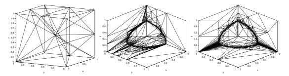
Figure 15: Example 5.3: the background tetrahedral mesh (left), the mesh structure on the coordinate planes from diagonal view for anisotropic (middle) and isotropic (right) linear interpolation.
