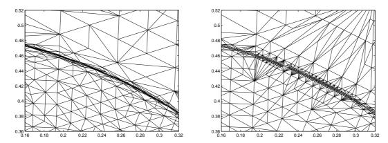
Figure 13: Example 5.2: the detailed mesh structure in the square  $[0.16, 0.32] \times [0.36, 0.52]$  for anisotropic (left) and isotropic (right) refinement.
