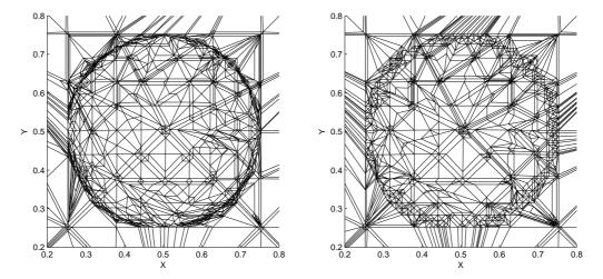
Figure 25: Example 5.6: the local mesh structure on z = 0.5 in the domain  $[0.2, 0.8] \times [0.2, 0.8]$ , for anisotropic (left) and isotropic (right) linear interpolation.
