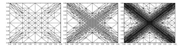
Figure 9: Example 5.1: the detailed mesh structure at the crossing of the two sharp layers in the square  $[0.45, 0.55] \times [0.45, 0.55]$  obtained after 8, 12 and 16 rounds of anisotropic refinement for the function f(x,y) (from left to right).
