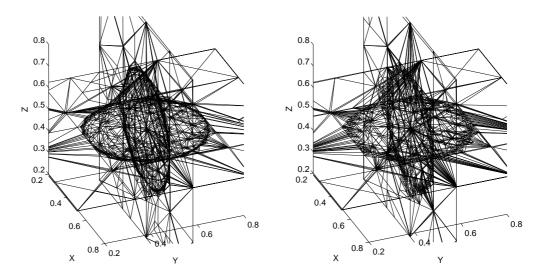
Figure 24: Example 5.6: the mesh structure on two slices for anisotropic (left) and isotropic (right) linear interpolation.
