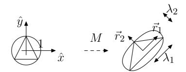
Figure 5: The transformation when the reference triangle is equilateral. The unit circle is mapped into an ellipse with directions  $\vec{r}_1$  and  $\vec{r}_2$ , the amplitude of stretching being  $\lambda_1$  and  $\lambda_2$ .
