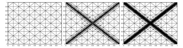
Figure 7: Example 5.1: the anisotropic refinement process for the function f(x,y). From left to right, the background mesh, the mesh obtained after 8 rounds of refinement, and the mesh after 16 rounds of refinement.
