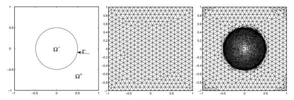
Figure 18: Example 5.4: the domain and interface (left), the background mesh with 505 nodes (middle) and the anisotropic mesh (right) with 6130 nodes.
