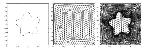
Figure 21: Example 5.5: the interface and domain (left), the background mesh with 505 nodes (middle), and anisotropic mesh (right) with 6130 nodes, using piecewise linear approximation.
