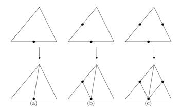
Figure 2: The three cases of refinement for one element in two-dimensional space.
