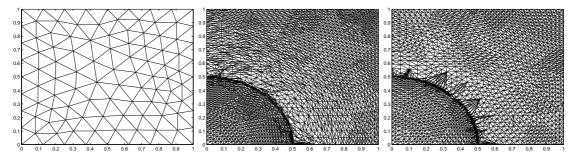
Figure 12: Example 5.2: the initial mesh with 105 nodes (left), the anisotropic mesh with 4141 nodes (middle) and the isotropic mesh with 4056 nodes (right) for linear interpolation.
