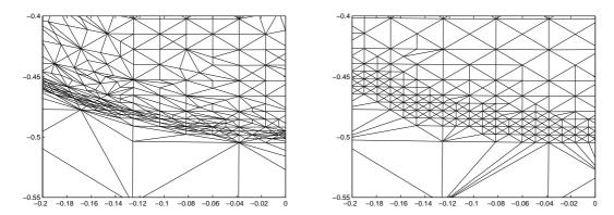
Figure 19: Example 5.4: the anisotropic (left) and isotropic (right) mesh structures in  $[-0.2,0] \times [-0.55, -0.4]$  using the ZZ error estimator.
