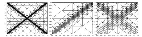
Figure 10: Example 5.1: the total mesh (left) and two detailed mesh structures in  $[0.6, 0.8] \times [0.6, 0.8]$  (middle) and  $[0.45, 0.55] \times [0.45, 0.5]$  (right) obtained after 12 rounds of isotropic refinement for the function f(x,y).
