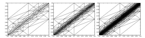
Figure 8: Example 5.1: the detailed mesh structure in the square  $[0.6, 0.8] \times [0.6, 0.8]$  obtained after 8, 12 and 16 rounds of anisotropic refinement for the function f(x, y) (from left to right).
