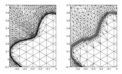
Figure 22: Example 5.5: the anisotropic (left) and isotropic (right) mesh structures in  $[-0.6,0] \times [-0.1,0.7]$ .
