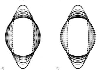
Figure 3: Surface diffusion flow  $(\delta=1,b=0,F=0)$  of an initial ellipse with a) and without tangential redistribution b). Numerical and redistribution parameters:  $n=100,~\tau=0.001,~\kappa_1=10.$  Time steps  $j=0,400,\cdots,2000$  are plotted using lines and grid points, while time steps  $j=200,600,\cdots,1800$  are plotted using lines.
