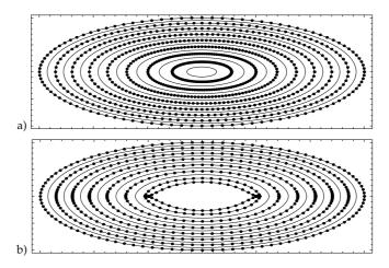
Figure 1: Affine invariant shrinking evolution of an initial ellipse  $(b=k^{1/3},\delta=0,F=0)$ ; a) with asymptotically uniform redistribution  $(\kappa_1=3)$ ; b) without redistribution. Numerical parameters  $n=100,\tau=0.001$ . Time steps  $j=0,200,\cdots,1400$  are plotted using lines and grid points, while time steps  $j=100,300,\cdots$ , up to j=1500 a); and j=1100 b) are plotted using lines.
