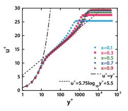
Figure 15:  $u^+$  distribution in the turbulent boundary layer.
