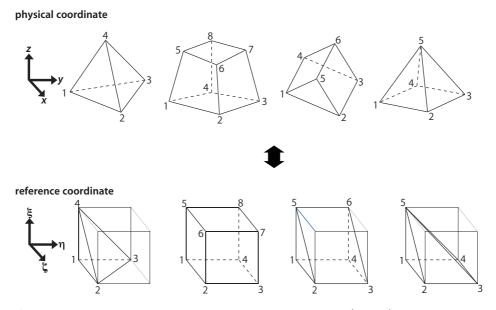
Figure 1: Schematic illustration of 3D mappings from the physical cell in (x, y, z) space to the reference cell in  $(\xi, \eta, \zeta)$  space.
