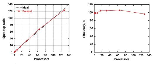
Figure 8: Speedup ratio. Dashed line represents the ideal speedup ratio, and solid line with symbols
