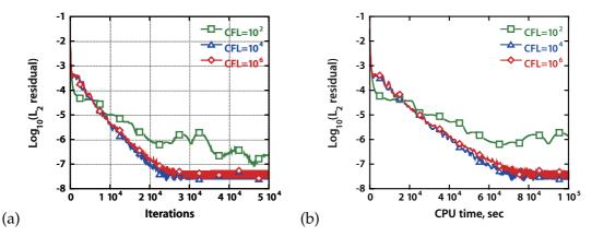
Figure 7: Convergence histories with different CFL numbers for flowfield over ONERA-M6 isolated wing in terms of; (a) number of iterations, and (b) CPU time.
