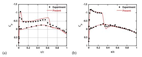
Figure 6: Pressure coefficient (Cp) profiles; (a) at 20% spanwise location, and (b) at 90% spanwise location. Symbols represent the Cp profiles from the experimental data and solid lines represent the computed Cp profiles.
