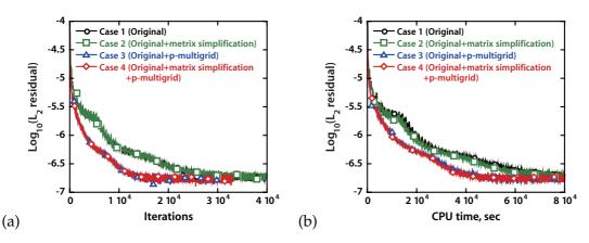
Figure 16: Convergence histories for the turbulent boundary layer flowfield over a flat plate in terms of; (a) number of iterations, and (b) CPU time.
