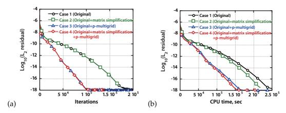
Figure 13: Convergence histories for the laminar boundary layer flowfield over a flat plate in terms of; (a) number of iterations, and (b) CPU time.
