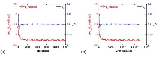
Figure 19: Convergence history for the flowfield over AGARD-B model in terms of; (a) number of iterations, and (b) CPU time.
