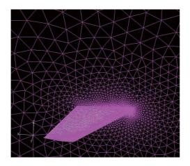
Figure 4: Unstructured mesh for ONERA-M6 isolated wing with 393,979 tetrahedral cells.
