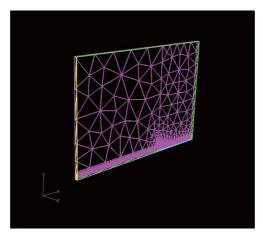
Figure 11: Hybrid mesh for the laminar boundary layer over a flat plate.
