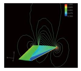
Figure 5: Pressure contours both on the wing upper surface and on the root plane.
