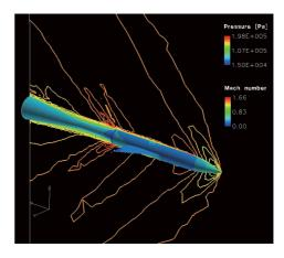
Figure 18: Pressure contours on the surface and Mach number contours on the root plane.
