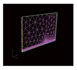
Figure 14: Hybrid mesh for the turbulent boundary layer over a flat plate.
