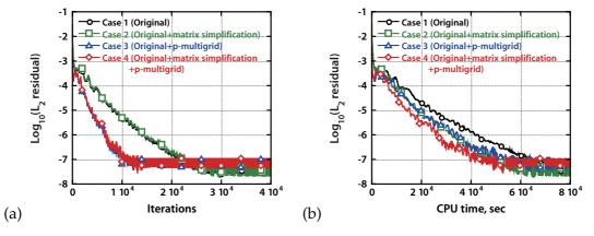
Figure 10: Convergence histories for the flowfield over ONERA-M6 isolated wing in terms of; (a) number of iterations, and (b) CPU time.
