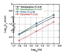
Figure 2: Error norms for various cell geometries are plotted in terms of mesh interval. The slope of the curve gives the spatial accuracy of the present scheme.
