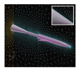
Figure 17: Unstructured hybrid mesh for AGARD-B model with 198,131 tetrahedral cells and 158,070 prismatic cells.
