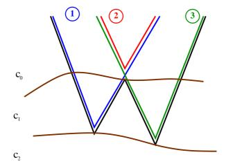
Figure 1: The sub-events of an internal multiple: the single reflections 1, 2 and 3 are arrivals in the data which satisfy the lower-higher-lower relationship in pseudo-depths z. The algorithm will construct the phase of the internal multiple (W shaped) by adding the phases of the deeper single reflections and subtracting the one of the shallow single reflection. The velocities for the three layers are represented by  $c_0$ ,  $c_1$  and  $c_2$ .
