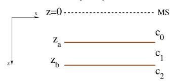
Figure 3: The model for the 1.5D example. The positive z direction points downward; the depths of the two interfaces are  $z_a$  and  $z_b$ ;  $c_0$ ,  $c_1$  and  $c_2$  are the velocities in the corresponding layers; MS denotes the measurement surface.
