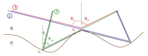
Figure 6: A 2D model with internal multiple reflections satisfying the time monotonicity in the vertical time but not in the total travel time.
