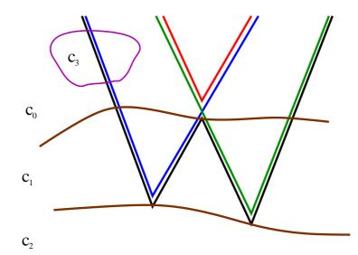
Figure 7: A 2D model with an internal multiple containing sub-events which do not satisfy the time monotonicity in either total traveltime or vertical time.
