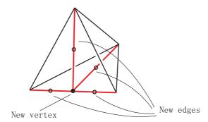
Figure 5: In a step of bisecting a tetrahedron, 4 new nodes will be created at most for a quadratic basis function.
