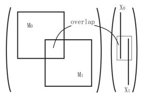
Figure 9: The matrices and vectors are stored locally on each processor, with the overlapping parts of the shared nodes of the neighboring sub-domains.
