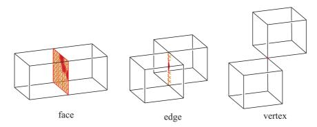
Figure 3: Three kinds of interface-mesh. The interface-meshes on the faces are triangular meshes, which are shared by two processors. The interface-meshes of the edges are 1-dimensional and shared by four processors. The interface-meshes on the vertices are shared by eight processes, which are trivial and never be changed during the refinements.
