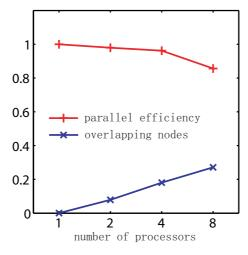
Figure 10: The parallel efficiency in  $H_2$  calculation.
