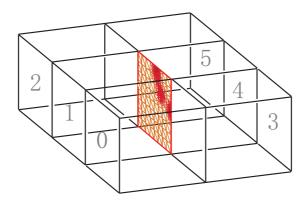
Figure 4: The neighboring sub-meshes of the interface-mesh.
