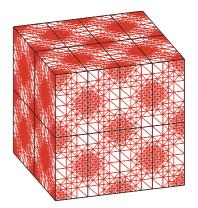
Figure 14: Domain subdivision of carbon nanotube with 16 ( $=4 \times 2 \times 2$ ) sub-meshes. The dark region shows the more refined part of the mesh where the nano-tube is located.
