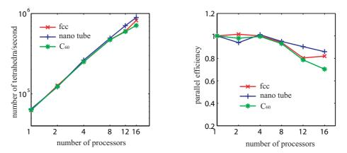
Figure 13: Number of tetrahedra/second and parallel efficiency versus number of processors.
