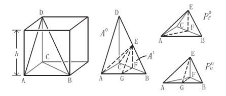
Figure 7:  $A^1$  type tetrahedra are obtained by 3 successive bisections of an  $A^0$  type tetrahedron. The right part of the figure shows the sequence of the bisections  $A^0 \rightarrow P_f^0 \rightarrow P_u^0 \rightarrow A^1$ .
