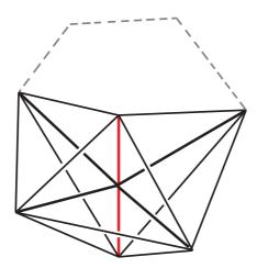
Figure 8: The refinement edge has n neighboring tetrahedron. The bisection of this edge will result in n+1 new edges, 2n new faces and n new tetrahedra.
