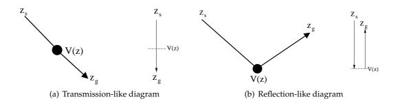
Figure 6: The figure displays the diagrams representing the time and the amplitude correction parts of the forward series in 1D: (a) Shows a time-corrector diagram. Downward propagation from source to the scattering point z and to the receiver. (b) Shows an amplitude corrector diagram. Downward propagation from source to the scattering point, z and upward propagation to the receiver.
