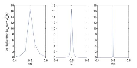
Fig. 4.3. Pointwise error in the cubic B-spline finite element approximation of the second derivative of the exact solution  $(|w_{xx}(x;0.5) - w_{xx}^N(x;0.5)|)$  for (a) N = 33, (b) N = 129, and (c) N = 1025 equally spaced finite element nodes. The error is essentially zero for all values of x not shown in the figures.
