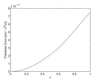
Fig. 4.1. The approximate pointwise sensitivity error for the homogenization approach using Hermite cubic finite elements with N = 7 equally spaced nodes and  $\alpha = 0.5$ . Note the scale on the vertical axis.
