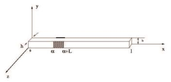
Fig. 2.1. Diagram of beam with a pair of piezoelectric patches of length L located on either side of the beam on the interval  $x \in [\alpha, \alpha + L]$ .
