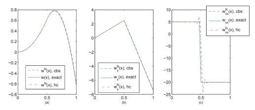
Fig. 4.2. The exact solution (3.5) of the model equation (3.3) for  $\alpha = 0.5$  compared with cubic B-spline (cbs) and Hermite cubic (hc) finite element approximations using 33 equally spaced nodes. Figure (a) compares the solution, and figures (b) and (c) compare the first and second derivatives, respectively.
