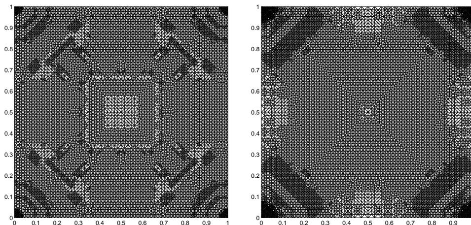
FIGURE 4. Example 1: Adaptively refined meshes. Left:  $\beta_1 = \beta_2 = \beta_3 = \beta_4 = 0.5$  (10 refinement steps, 17760 elements). Right:  $\beta_1 = \beta_2 = \beta_3 = \beta_4 = 0.99$  (10 refinement steps, 19744 elements).
