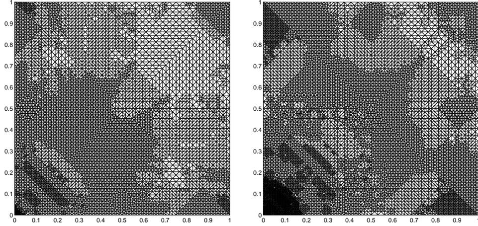
FIGURE 3. Example 1: Adaptively refined meshes. Left:  $\beta_1 = 0.5$ ,  $\beta_2 = \beta_3 = \beta_4 = 0.0$  (12 refinement steps, 11768 elements). Right:  $\beta_1 = 0.99$ ,  $\beta_2 = \beta_3 = \beta_4 = 0.0$  (13 refinement steps, 16362 elements).
